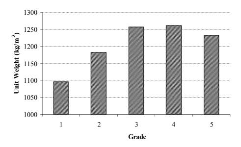
Figure 4. Unit weight of 28 aged PLWAC
