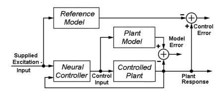
Figure 3. Architecture of control system based on reference model
