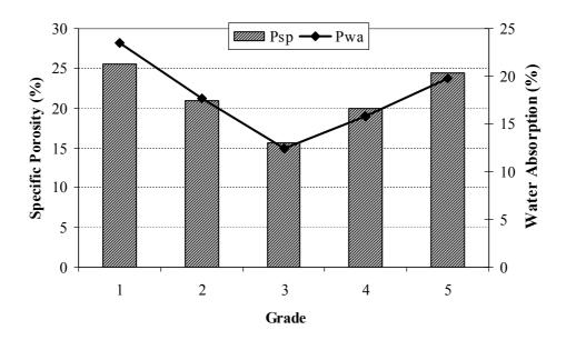
Figure 5. Specific porosity (sp) and water absorption (wa) of 28 aged PLWAC
