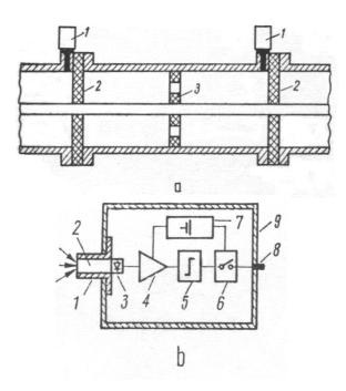
Figure 3. Light emission based fault location method applied to a capsulated SF<sub>6</sub> compartment
