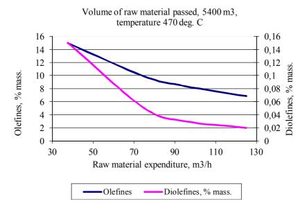
Figure 7- Change of concentration of olefines and diolefines depending on temperature and the expenditure of raw material at 5,4 thousand m<sup>3</sup> of raw material passed (about 3 days of plant work)
