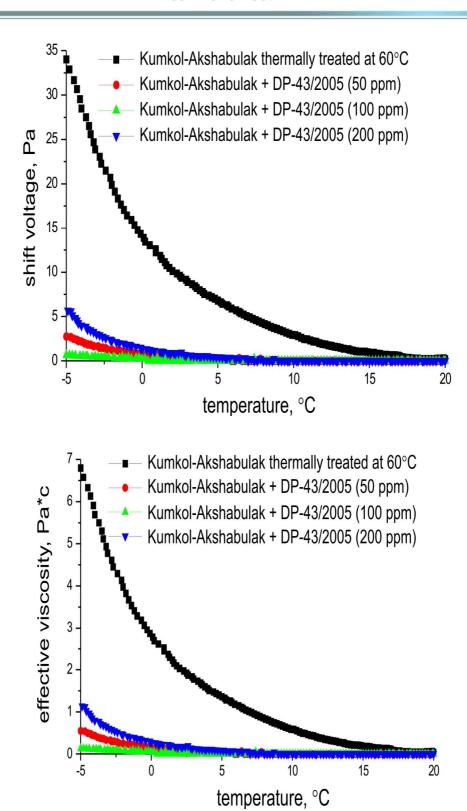
Fig. 1 Shift voltage (a) and effective viscosity (b) depending on temperature for the Kumkol/Akshabulak oil mix (60:40 vol.%) after treating by heat and the DP-43/2005 dopant, respectively.
