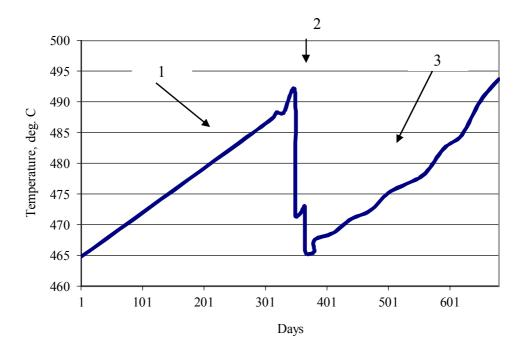
Figure 12. - Temperature of an input of raw material at the organization of continuous work of hydrogenation reactors
