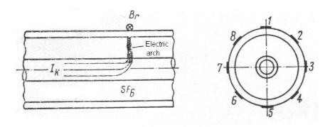
Figure 2. Magnetic field based fault location method applied to a capsulated bar system
