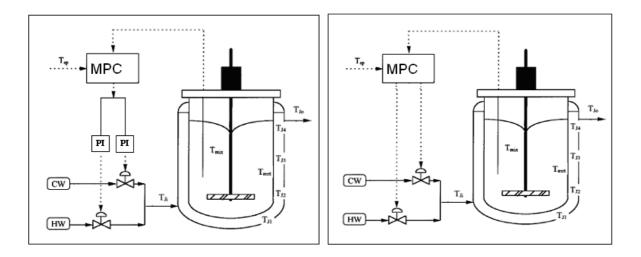
Fig.2. The implemented reactor temperature control systems.
