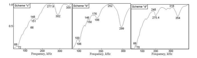
Figure 7. Frequency response of polymeric composite specimen (experimental data – explanation in text)
