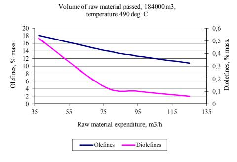
Figure 6- Change of concentration of olefines and diolefines depending on temperature and the expenditure of raw material at 184 thousand m<sup>3</sup> of raw material passed (more than days of plant work)
