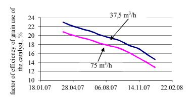
Figure 2. A degree of the catalyst use in dependence on loading on raw material and time of the catalyst operation
