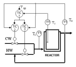
Fig. 1. Reactor temperature control system
