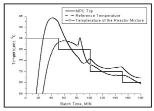
Fig.5. Step changing temperature reference.
