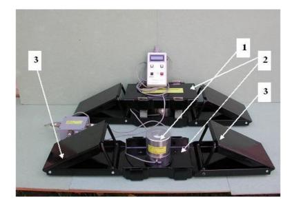
Figure 3. Prototype used for the mass measurement of light vehicles
