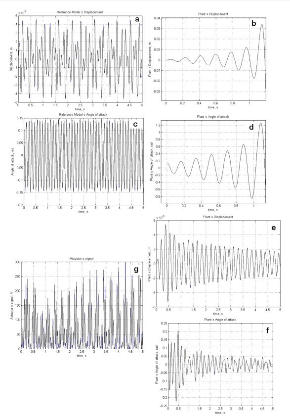
Figure 8. The time charts of displacement and angle of attack at airflow speed 60 m/sec:
