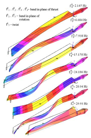
Figure 6. First vibration modes of model blade
