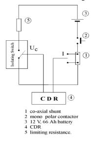
Figure 3. Block diagram of measuring and recording contact resistance
