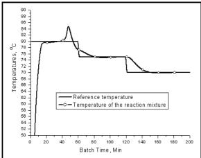
Fig.9. Step changing temperature reference.
