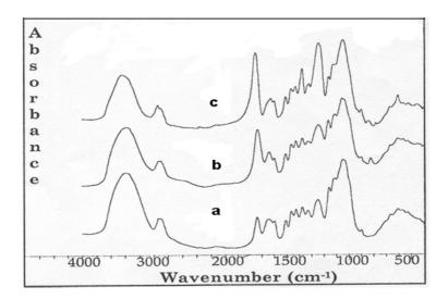
**Fig. 1.** FTIR spectra of esterified and control wood: (a) control, (b) modified with maleic anhydride and (c) modified with acetic anhydride.
