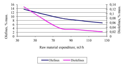
Figure 5 - Change of concentration of olefines and diolefines depending on temperature and the expenditure of raw material at 184 thousand m<sup>3</sup> of raw material passed (more than days of plant work)
