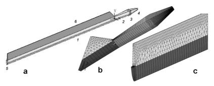
Figure 5. The simplified rotor blade finite-element model a - full view; b - near root; c - near tip
