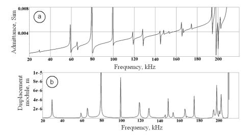
Figure 9. Frequency response of admittance (a) and the surface point's displacement modulus for studied polymeric composite specimen (simulation results)
