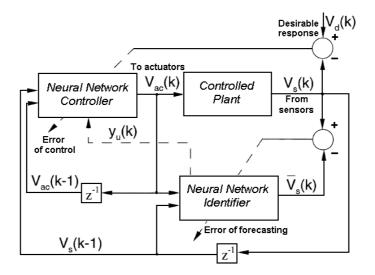
Figure 2. Neural network architecture of system for structure's vibration adaptive control (after Valoor et al., 2001)
