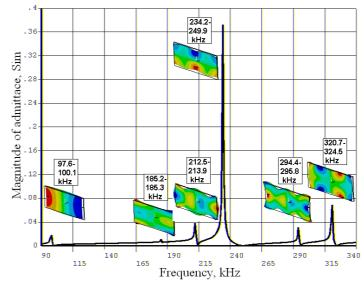
Figure 3. The frequency response of piezoelectric plate's admittance (FEM - simulation results)
