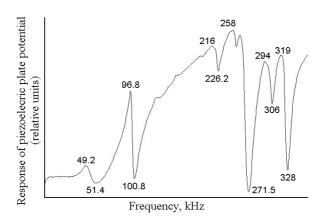
Figure 1. The frequency response of piezoelectric plate potential (experimental data) mechanical boundary conditions
