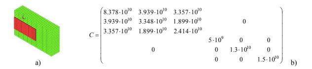
Figure 8. FE – model of specimen with attached piezoelectric elements (a) and stiffness matrix for used orthotropic composite material (b)
