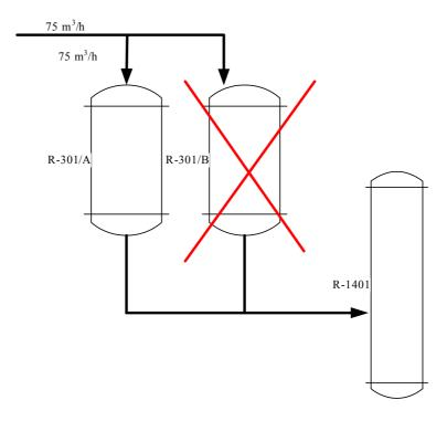
Figure 11- monoreactor operating mode
