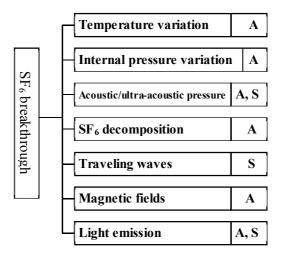
Figure 1. The effects of SF<sub>6</sub> breakthrough and their use for fault location
