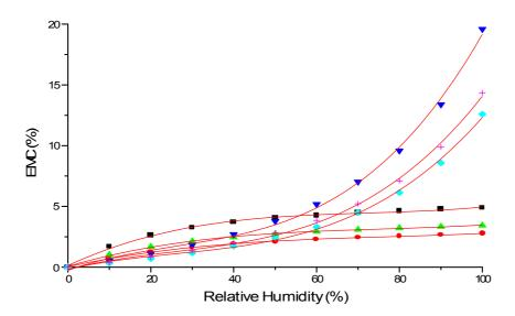
**Fig. 3.** Polymolecular adsorption isotherms for unmodified (▼), modified with acetic (♦), maleic (+) anhydride elm wood and monomolecular adsorption isotherms for unmodified (■), modified with acetic (●), maleic (▲) anhydride elm wood.
