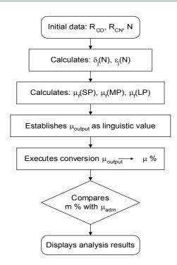
Figure 5. Block diagram of the algorithm used for establishing the period of predictive maintenance of SIT electric contacts
