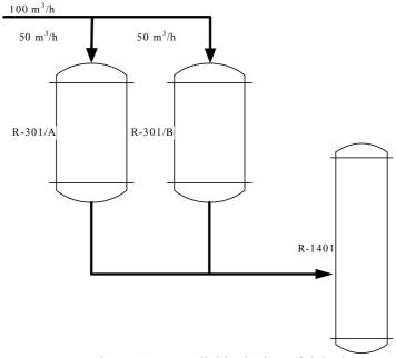
Figure 10. - parallel inclusion of dehydrogenation reactors
