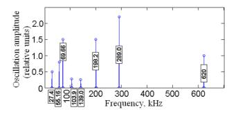
Figure 6. Frequency response of polymeric composite specimen (experimental data obtained by displacements optical meter)
