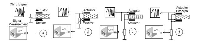
Figure 4. Electrical circuits for specimen's excitation on different oscillation natural modes
