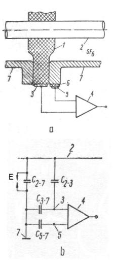
Figure 4. Partial discharges detection method applied to a capsulated SF<sub>6</sub> installation
