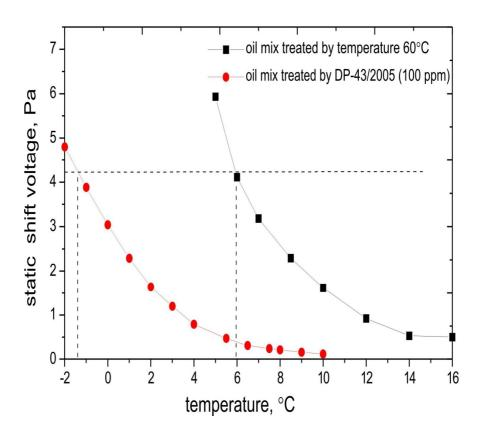
Fig. 2. The static shift voltage depending on temperature for the Kumkol/Akshabulak oil mix (60:40 vol.%) after treating by heat and the DP-43/2005 dopant, respectively.
