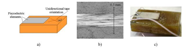
Figure 5. Composite specimen for determination of elastic constant by dynamic test: a – schematic view; b – magnified transversal cross-section normal to largest plane; c – snapshot of specimen with installed piezoelectric elements
