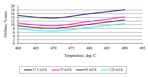
Figure 4. - Change of concentration of olefines depending on temperature and expenditure of raw material at 184 thousand m<sup>3</sup> of raw material passed (more than days of plant work)
