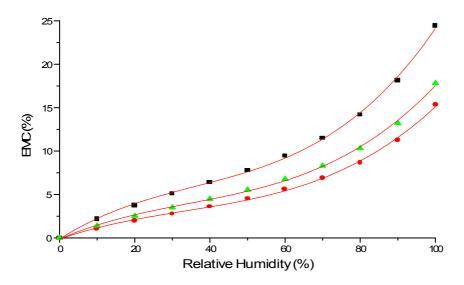
**Fig. 2.** Adsorption isotherms for unmodified (■), modified with acetic (●) and maleic (▲) anhydride elm wood.
