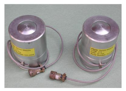
Figure 2. Cylinders with differential piston (measuring transducers)
