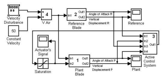
Figure 7. Simulink - model of neural network system for vibration damping of rotor blade finite element model
