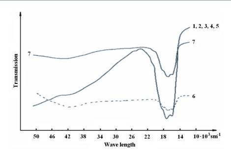
Fig. 3. Diffuse reflection spectra of CoO (5 % mas.) - γ-Al<sub>2</sub>O<sub>3</sub> system after processing by initial reactants: 1 – fresh catalyst; 2 – after processing in CO<sub>2</sub>; 3 – after processing by oxygen of air;
