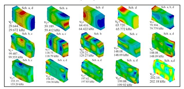
Table 2 - The natural modes of composite specimen's oscillation (simulation results).
