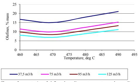
Figure 3. - Change of concentration of olefines depending on temperature and expenditure of raw material at 5 thousand m<sup>3</sup> of raw material passed (about 3 days of plant work)
