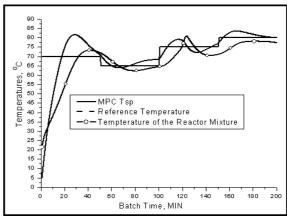
Fig.6. Step changing temperature reference.
