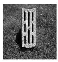
Figure 2 Masonry blocks produced with pumice LWA
