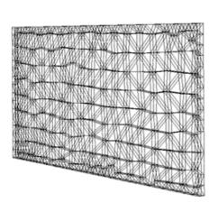
Figure 2. The finite element meshing of piezoelectric plate
