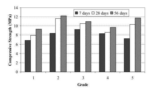
Figure 3 Compressive strength of PLWAC in different ages and gradations
