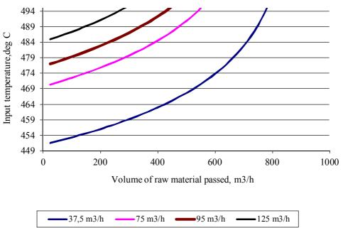
Figure 9. -Change of an input temperature in a dehydrogenation reactor at the various raw material expenditure
