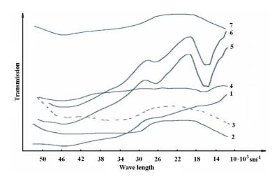
Fig. 2. Diffuse reflection spectra of NiO (10 % mas.) -  $\gamma$ -Al<sub>2</sub>O<sub>3</sub> system after processing by initial reactants: 1 – the fresh catalyst; 2 – after processing in CH<sub>4</sub>; 3 – after processing in mix CH<sub>4</sub> + CO<sub>2</sub>; 4 – after processing in mix CH<sub>4</sub> + air; 5 – after processing in CO<sub>2</sub>; 6 – after processing by air oxygen; 7 – after processing in mix CH<sub>4</sub> + CO<sub>2</sub> + air
