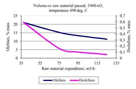
Figure 8- Change of concentration of olefines and diolefines depending on temperature and the expenditure of raw material at 5,4 thousand m<sup>3</sup> of raw material passed (about 3 days of plant work)
