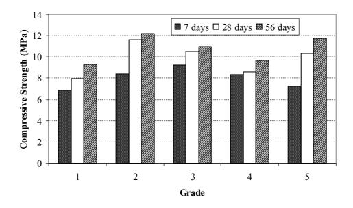
Figure 3 Compressive strength of PLWAC in different ages and gradations
