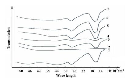
Fig. 1. Spectra diffuse reflection of NiO (5 % mas.) - γ-Al<sub>2</sub>O<sub>3</sub> system after processing by initial reactants: 1 – fresh catalyst; 2 – after processing in CH<sub>4</sub>; 3 – after processing in mix CH<sub>4</sub> + air; 4
