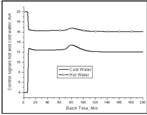
Fig. 12. Control inputs of the polymer reactor.
