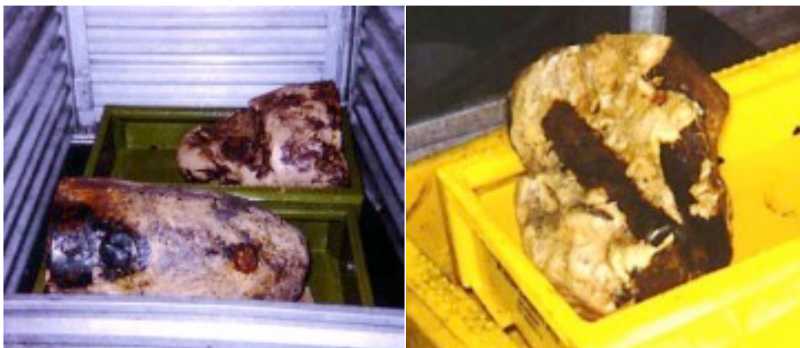
Fig. 3 Lumps of solidified sulphur iperite fished out with hooks
