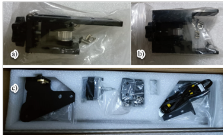
Fig. 3. Mechanical improvement parts a) X axis tensioner b) Y axis tensioner c) Dual Z axis trapez screw
