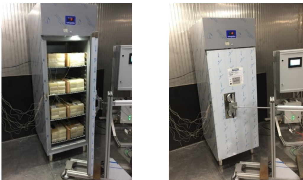
Fig. 9. Door opening and closing in commercial refrigerator prototype test application.
