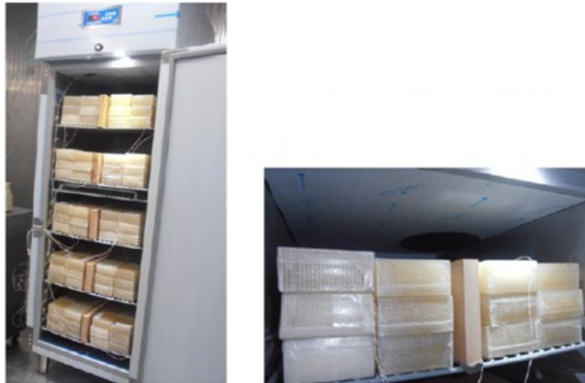
Fig. 8. The test packages in the evaluation process of the cooling performance in the commercial refrigerator prototype.
