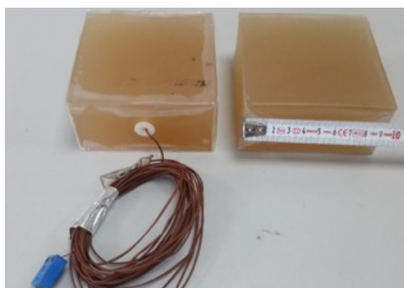
Fig. 7. The photograph of the test packages (50x100x100 mm / 500 g.).
