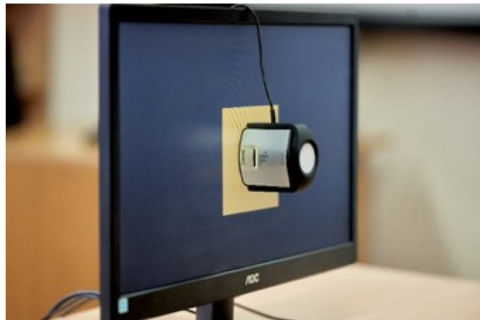
Fig. 3. Measurement of the display color parameters using X-Rite i1Display Pro
