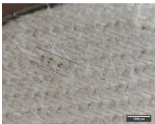
Picture 1 Failure point of denim sample in flat abrasion
