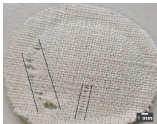
Picture 4 Abrupt failure of hemp canvas in flat abrasion
