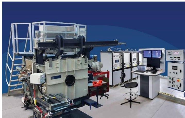
Fig. 2. Experimental electron beam welding workplace for research on the welding of Cr-Mo steels
