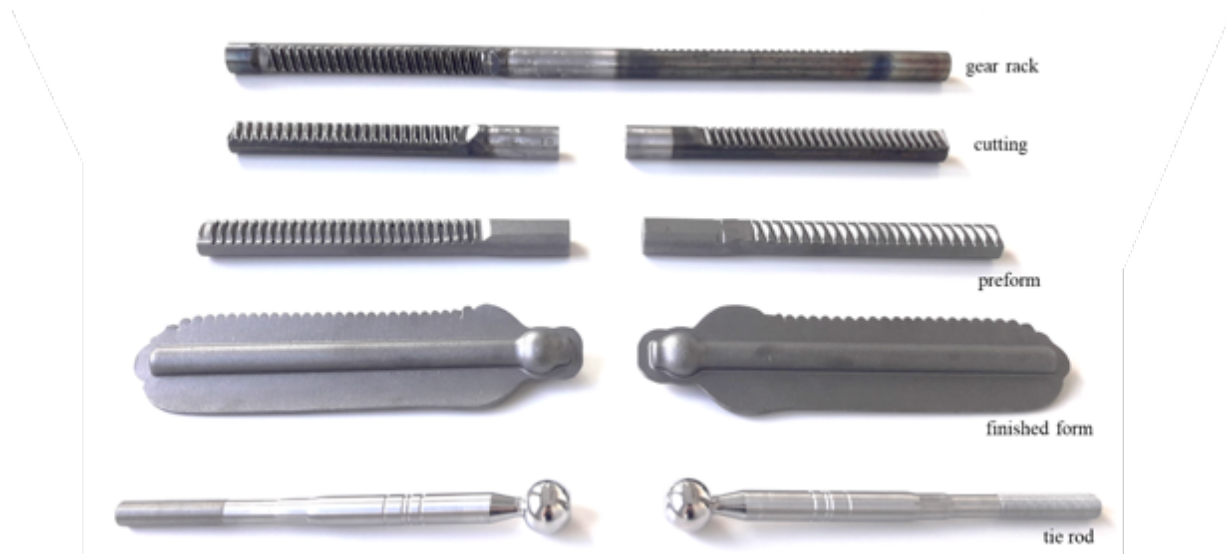
Fig. 9. Demonstrator EKODA, repurposing of one gear rack to two tie rods
