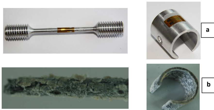
Fig. 4. a) Cylindrical and C-ring SCC specimens before and b) after an SCC test, conducted at the AUTH Corrosion Center.
