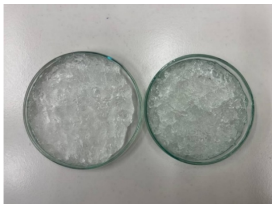
Fig. 1. SAPs used in the assays – SAP1 (left side) and SAP2 (right side) – product after absorption of water. Source: our elaboration
