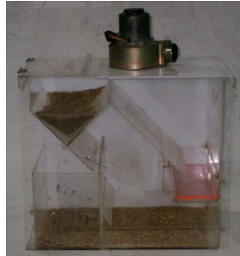
Figure 6. Vertical winnowing separator (air velocity of winnowing section is 6.90 m/s)
