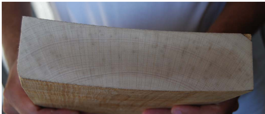
Fig.1. Darker inner part of a beech plank, known as “sandwich” effect, effect” combined with darker spots on all transverse section
