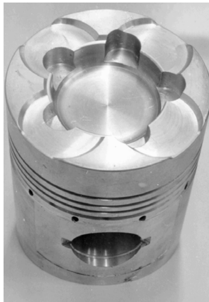
Fig. 3. Bowl in piston combustion chamber with turbulence generator (Kutenev et. al., 1998)
