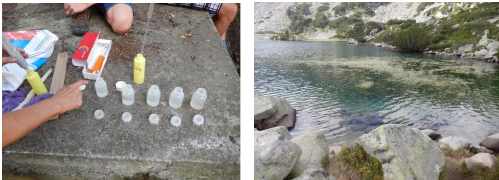
Fig. 2. Fixing the dissolved Oxygen (left) in the water from lake with eutrophication (right)
