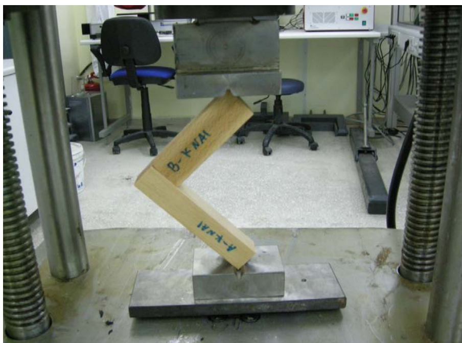
Fig. 1. Bending test of impregnated beech wood corner joints.
