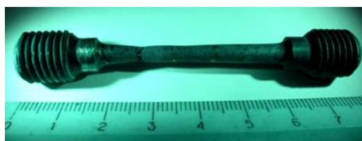
Figure 4. Test sample after high temperature creep-rupture test
