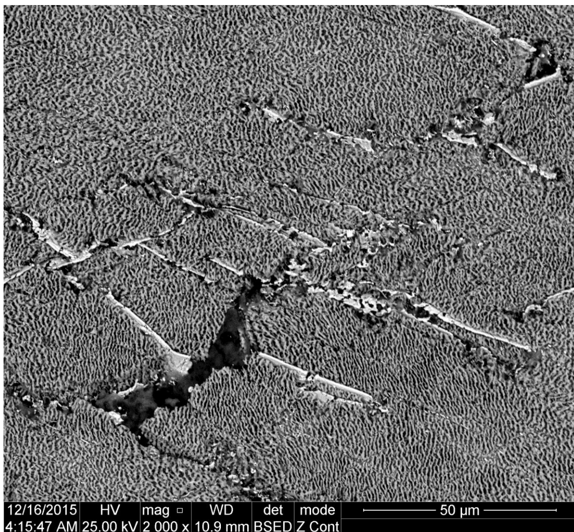
Figure 5. Single-crystal test specimen fracture zone along the TCP-phases accumulation.
