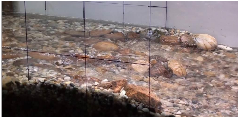
Fig. 6. W – rock weir / discharge ( Q_{scale} = 10,27 \text{ l.s}^{-1} , Q_{real} = 3,247 \text{ m}^3.\text{s}^{-1} )
