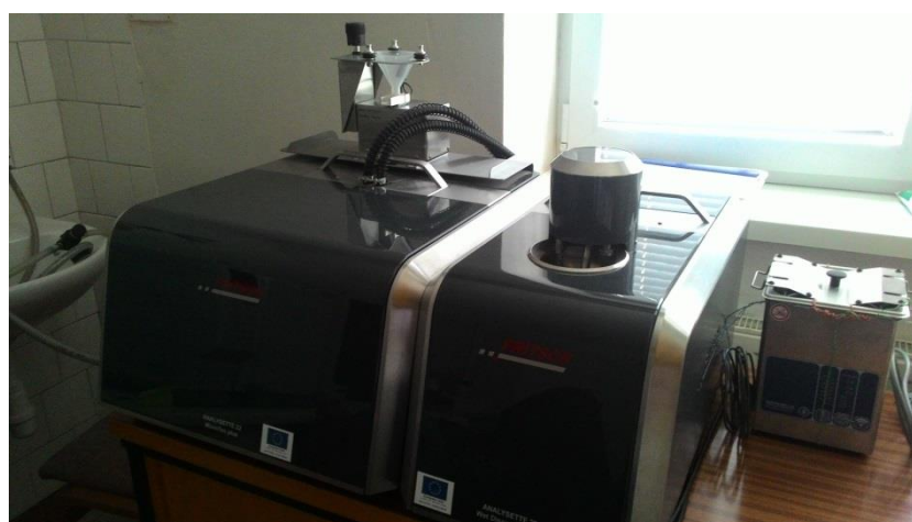
Fig. 2. ANALYSETTE 22 MicroTec plus: measuring unit and wet dispersion unit, ultrasound (Source: Šinkovičová, 2016)
