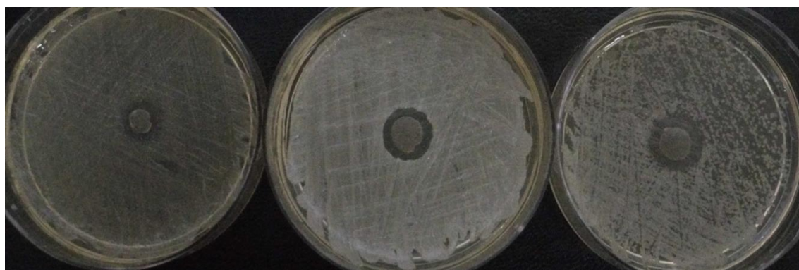
Figure 3. Photograph of antimicrobial test result of agar/Ag film against E. coli (left), S. aureus (middle) and C. albicans (right)
