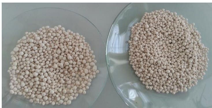
Fig. 1. Zeolite granules (left) and zeolite granules modified by \text{TiO}_2 (right)
