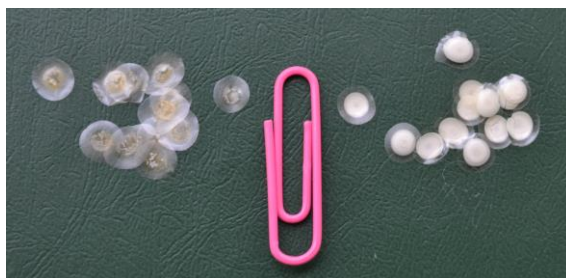
Fig. 6. The multicomponent reagent 'Enzymolum' is a flake of dried gel, diameter 6–7 mm; dry weight 1.5 \pm 0.2 mg.
