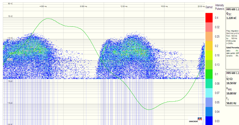
Fig. 13. PRPD pattern of the XLPE thermally aged samples (30 days_125 °C at 10 kV (Q = 1.2nC))
