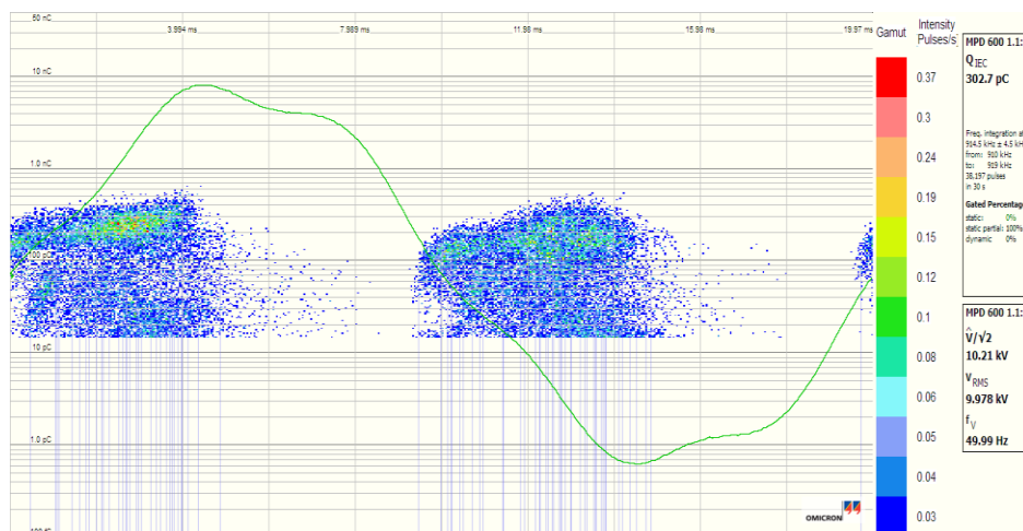
Fig. 14. PRPD pattern of the EPR thermally aged samples (30 days_125 °C at 10 kV (Q = 302 pC))
