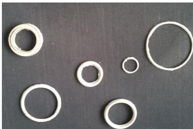
Fig. 1. O-rings from nanocomposites based on natural rubber, plasticized starch, precipitated silica and layered clay
