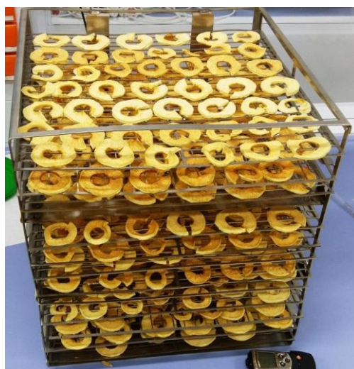
Fig. 4. The apple rings dried in the 500mm size dehydrator; herewith the rings were allocated on the greatly perforated trays
