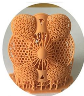
Fig. 5. Product demonstrating the advantages of three-dimensional printing in the production of complex parts
