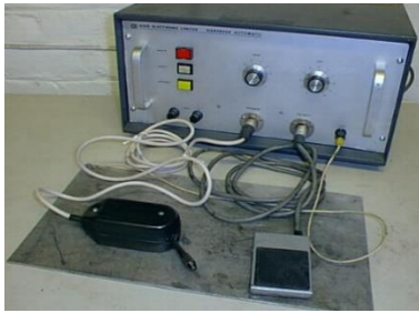
Fig. 1. Device for manual electrical discharge deposition with vibrating electrode.
