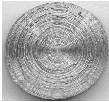
b) initial invar after rough turning, initial: R_a=10.7 , R_z=30.2 , R_q=12.24 , R_t=29.64
