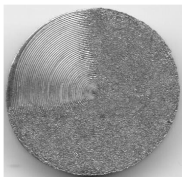
a) Inconel surface after pure turning, and after ESD at E=0.04 J: initial R_a=3.2 , coating R_a=3.55
