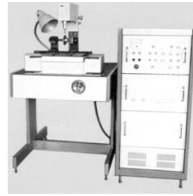
Fig. 2. Machine Elfa 541 for contactless LESD.
