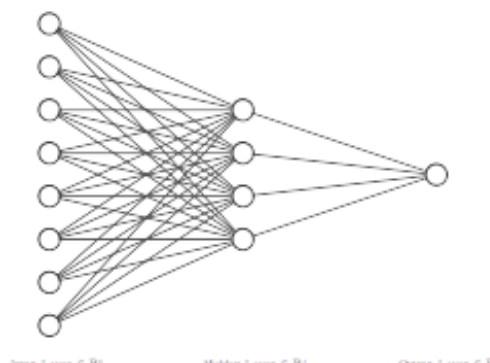
Fig. 1. multilayer perceptron (MLP) with one hidden layer
