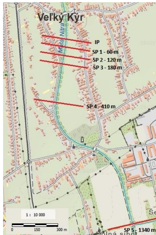
Figure 2. Location of the tracer injection and sampling points on the Malá Nitra River
