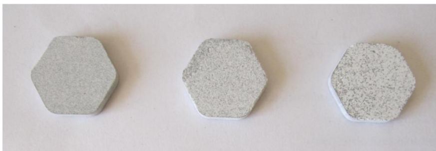
Figure 1. Hexagonal form of the compacts of \text{Al}_2\text{O}_3 / SiC composites for EMS testing
