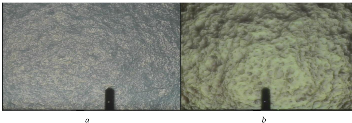
Fig. 1. The optical images of the organosilicate weather-resistant coating surfaces of «hot» (a) and «cold» curing (b), aminopropyltriethoxysilane as a hardener. Label – 25 microns [7]
