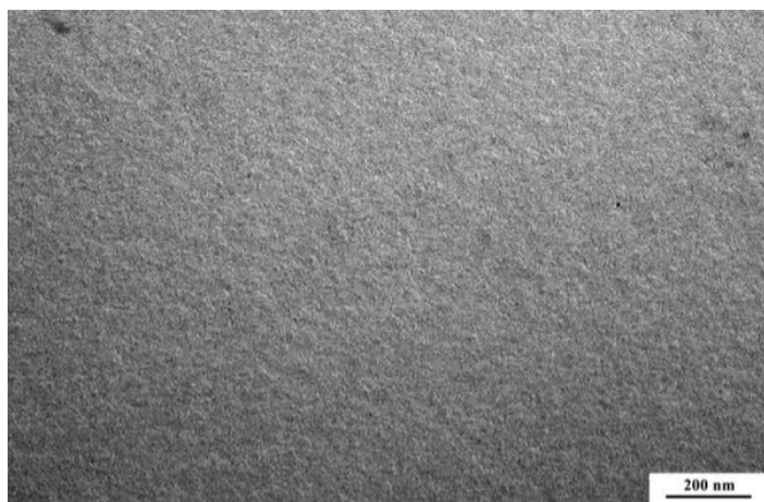
Fig. 2. TEM micrograph of initial PET film surface (5 \mu\text{m} thickness).
