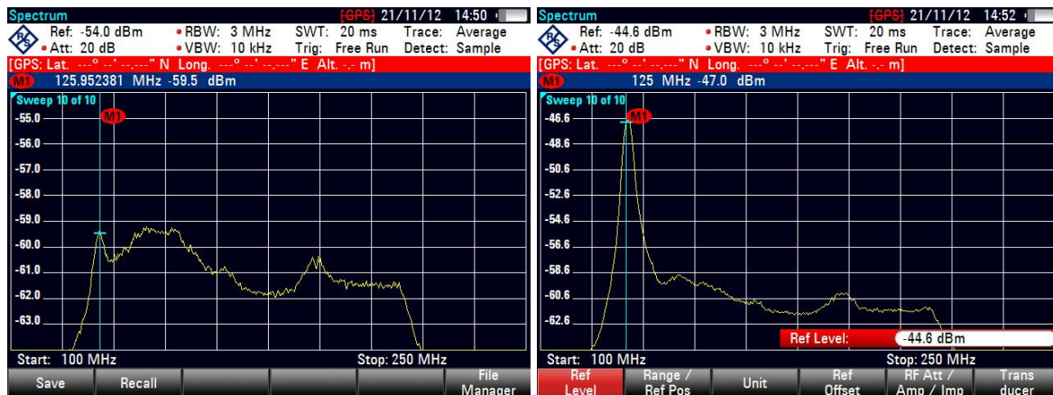
Fig. 6. Received GPS satellite down-converted signals in transient mode: on left – before entering RT-16 antenna pointing maximum; on right – entering RT-16 antenna pointing maximum.
