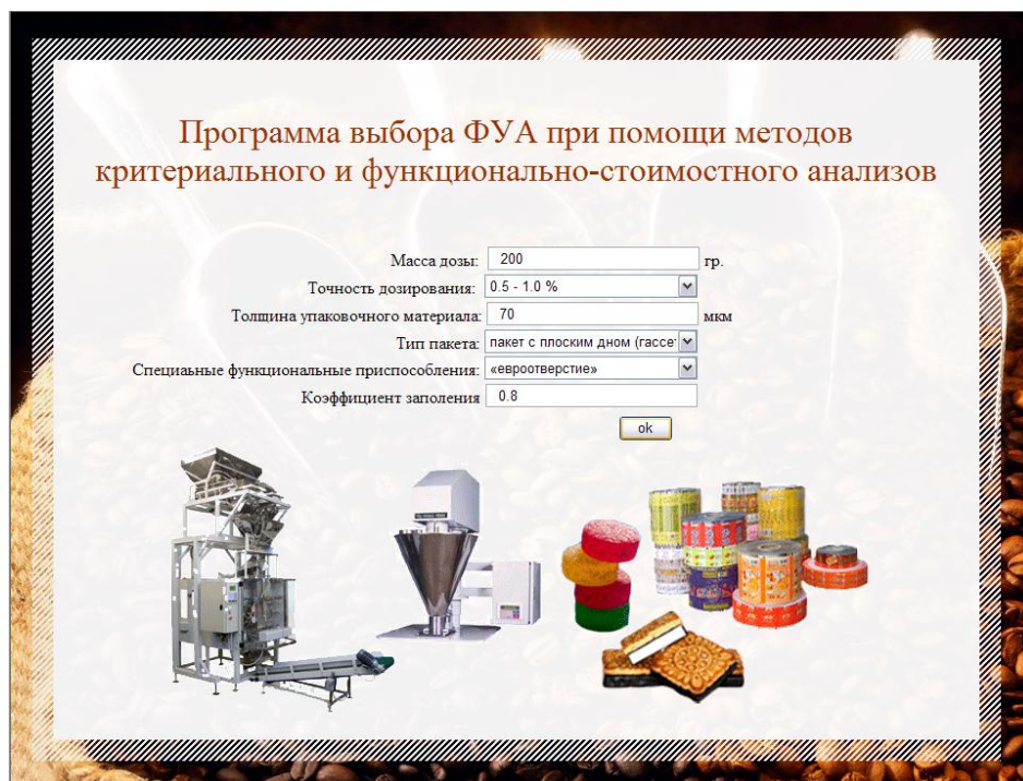
Fig. 3. The dialog box №2 (inputting of the dose of mass, the measure accuracy, the thickness of packaging material, the percent of package filling with product (a mark to space ratio) and choosing a type of package).
