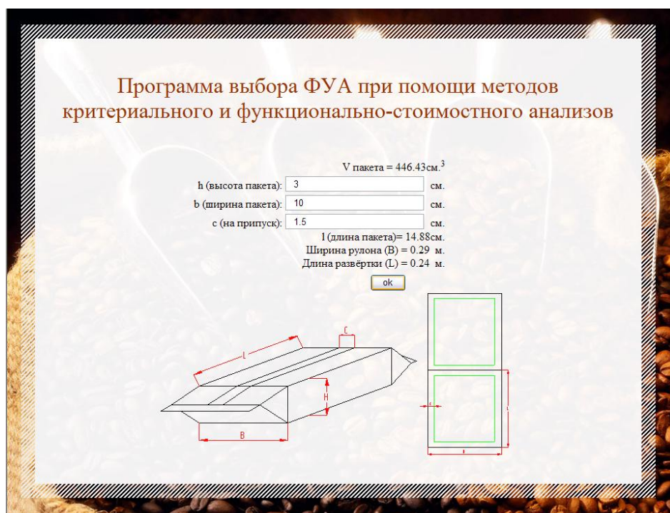
Fig. 4. The dialog box №3 (inputting of the required package high, the width and allowances; program calculates the package length, the width of package film and the length of package drawing).
