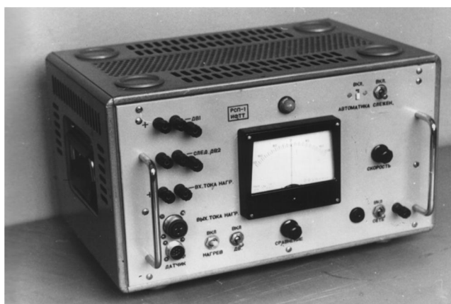
Fig. 10. Appearance of an appliance for a control of speed of tape passage
