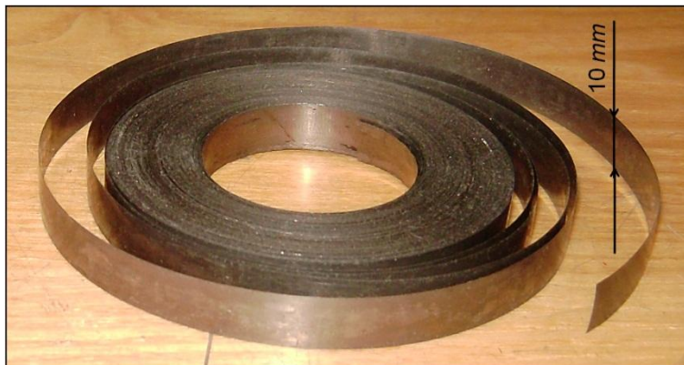
Fig. 20. Segment of multilayer Nb/D16 tape
