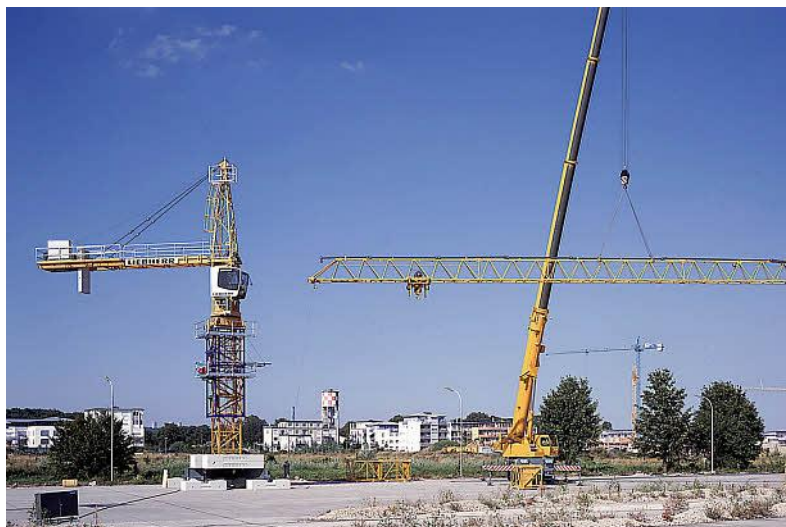
Fig. 5. An example High-top-EC-H: builder (Source: Liebherr 2006a, accessed February 13 2012).
