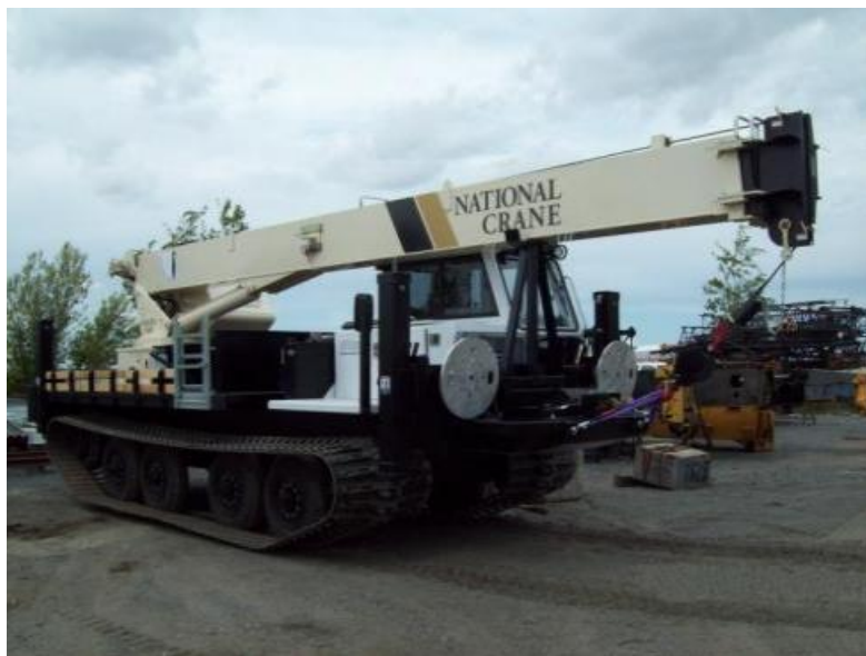
Fig. 2. An example Crane for soft terrain (Source: Pragotechnik 2011c, accessed February 12 2012).
