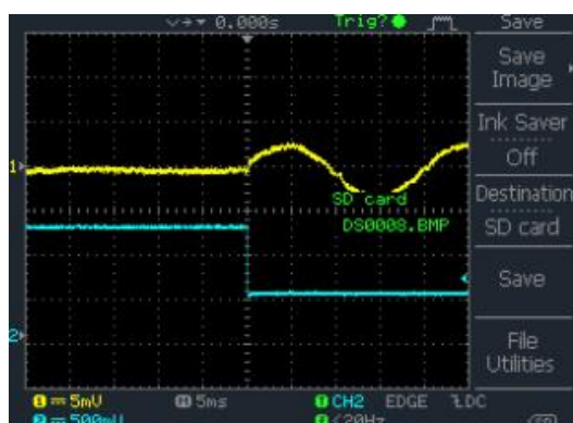
Fig. 17. Oscillograms of the currents in DAVR at a commutation angle 135^\circ and RC-load.
