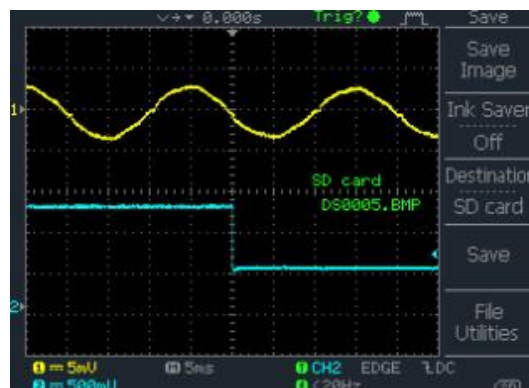
Fig. 16. Oscillograms of the currents in DAVR at a commutation angle 45^\circ and RC-load.
