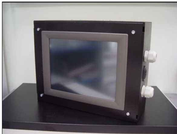
Fig. 3. Computer operator panel
