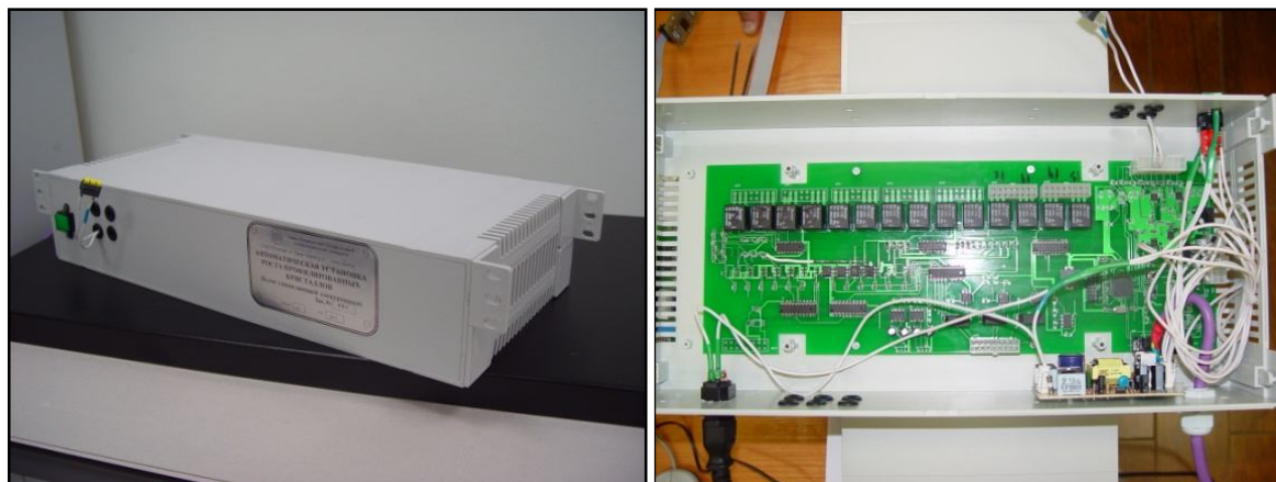
Fig. 4. control board, based on the microcontroller Atmega 128 A
