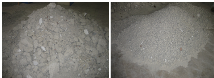
Figure 1. Cracked and sieved waste concrete in laboratory
