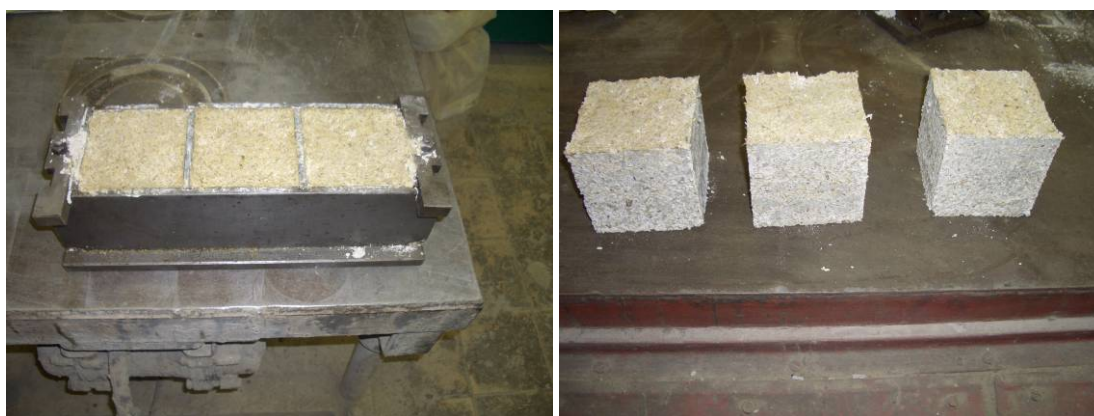
Figure 5. Test specimens in a mould and after removal from the mould.
