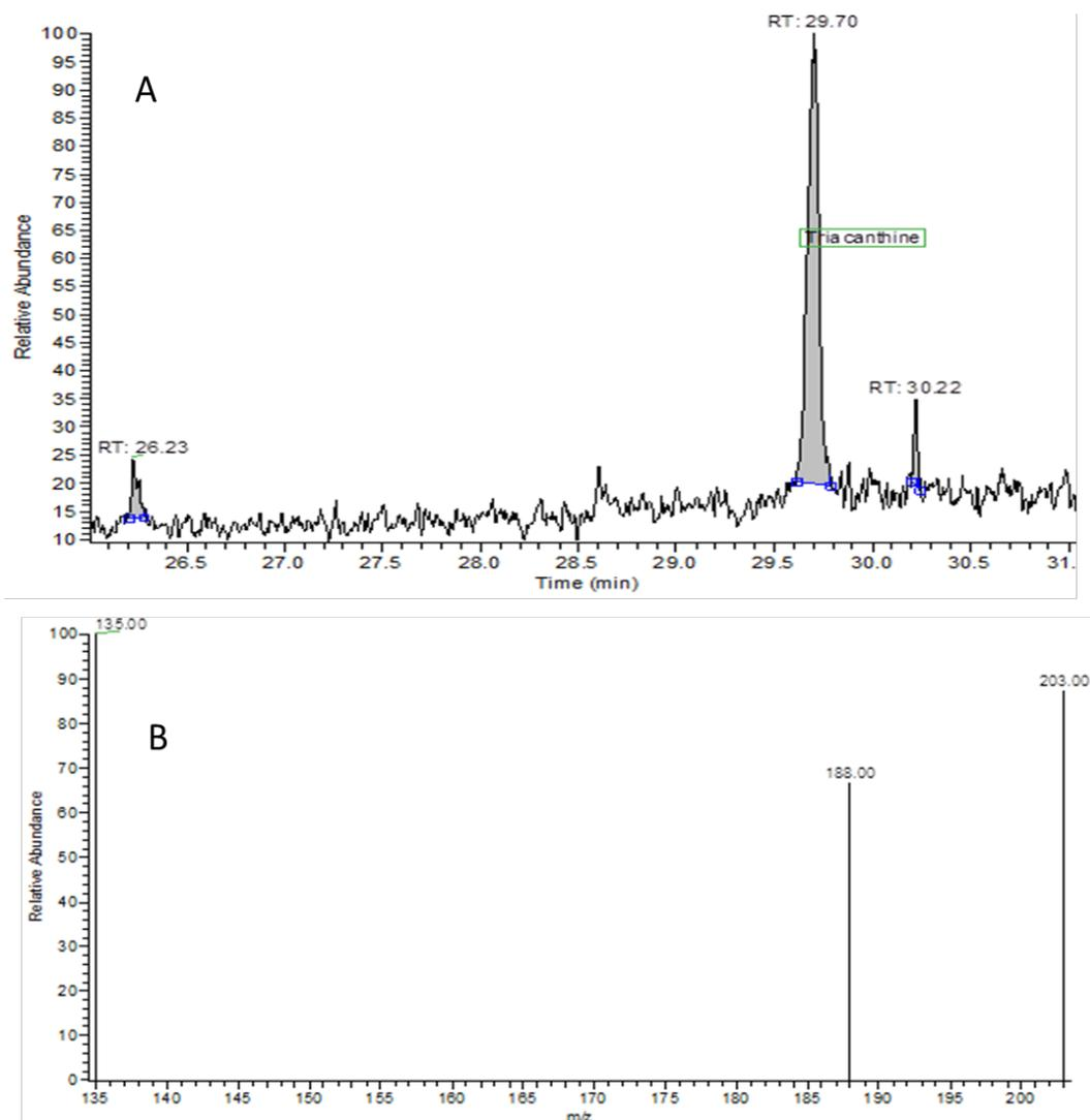
Fig. 4. Chromatographic profil and mass spectrum of alkalod triacanthine. A: GC chromatogram of alkaloidal fraction of *Gleditsia triacanthos*. The retention time of triacanthin is 29.70 min. B: Mass spectrum of triacanthine. The characteristic ions are: m/z 135 (100), m/z 188 (62), m/z 203 (71)
