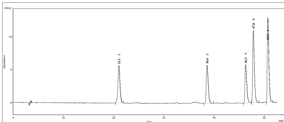
Fig.5. HPLC profile of standart compounds: 1-chlorogenic acide; 2-rutin; 3-luteolin; 4-quercetin; 5-apigenin
