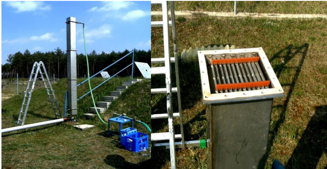
Fig 1. Pilot-scale aeration tower for radon removal (Photo - Munka)
