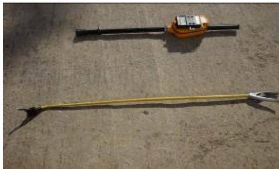
Figure 6. Radiation measuring device (on the top of the photograph). Clamp for handling of radioactive sources (on the bottom of the photograph)
