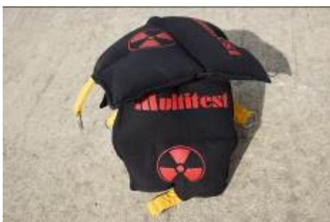
Figure 9. Bags with lead spheres for radiation protection of the sources
