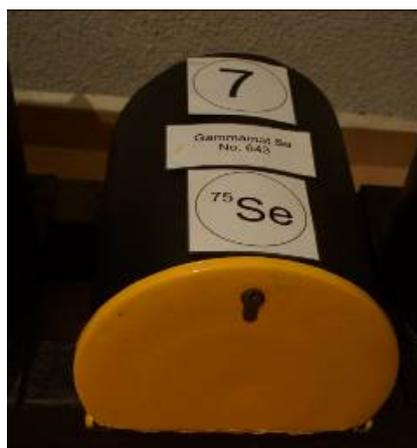
**Figure 16.** Sample of a container, where the found radioactive sources were placed for temporary storage
