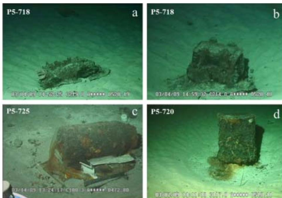
Figure 4. Examples of corrosion skirt features observed: (a) bomb casing, (b) ammunition box, (c) aerial depth bomb, (d) discarded depth charge (Silva & Chock, 2016).
