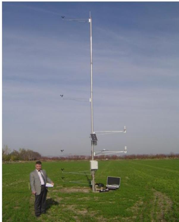
**Figure 1.** Agrometeorology station established in the winter wheat field.
