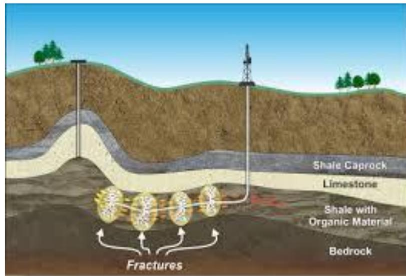
**Fig 2.** Method of hydraulic fracturing
