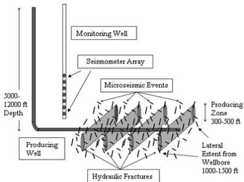
Fig 5. Schematic diagram of the development of hydraulic fractures and micro-quakes in a succession of fractal wells
