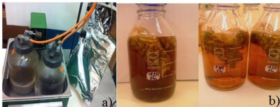
**Fig. 4.** a) Setup of anaerobic digestion of pretreated samples, b) Experiments of biomass alkaline soaking
