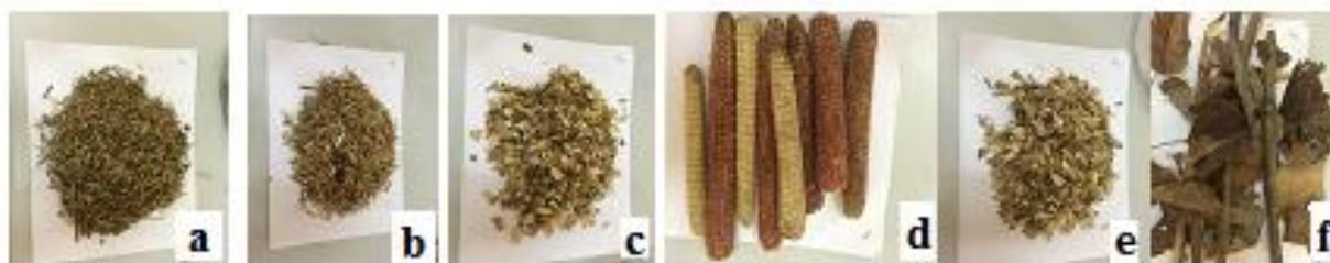
**Fig. 1.** Samples of all raw materials used for the experiments in raw: a) alfalfa, b) wheat straw, c) corn straw, d) corncob, e) a mixture of leaves and f) thin and dry wooden sticks.
